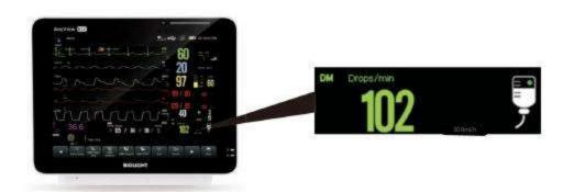
The DM module can control the drip rate all the time during infusion. When the infusion is complete, the module will clamp the infusion tube to prevent blood reflux.
