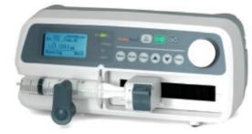
Applicable syringe: 5, 10, 20, 30, 50/60 ml, increments of 0.01 ml/h for flow rate, bolus flow rate, KVO flow rate
